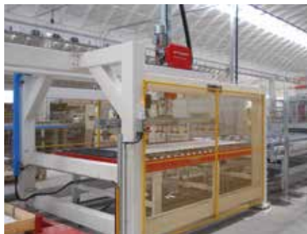
LOADER FROM WOODEN BOXES
