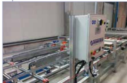
*The small dimensions and the software control make it possible to turn large formats as well in a limited space even at high speeds, and thanks to the jogger function, the turned*
