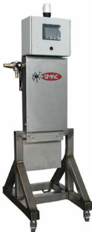
*to automatic control devices at continuous cycle with automatic recirculation. The machine is designed to adapt to the existing equipment in the glazing line, thus avoiding the need to purchase new equipment and other dedicated to the device. The device can automatically controls two dosing pumps for the feeding of chemical additives or color bases.*
