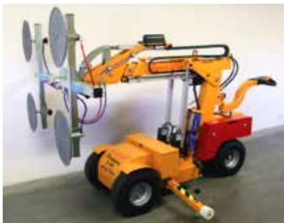
**The Smartlift SL series manipulators** are the ideal way to lift loads outdoors or indoors, up to 608 kg at a height of about 4 meters. Equipped with electronic brake and double vacuum circuit, they guarantee easy operation even in tight spaces. The Smartlift is easily transportable on vans or trailers. The fork equipped with suction cups moves in all directions to ensure maximum flexibility of use
