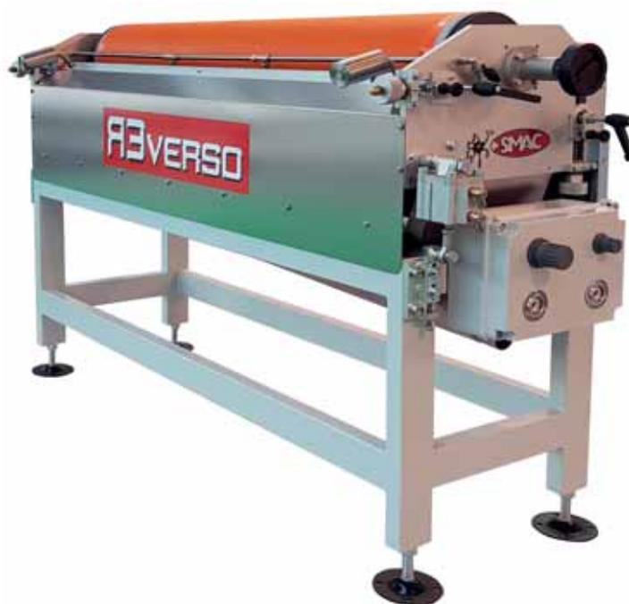
The management is completely automatic, through an electrical control panel with PLC and programming keyboard. The DSR machine can be equipped with a separated feeding container (model CF) to increase the production autonomy. In case of production with glue digital printing, the system could be completed with the suction device model CGA, complete with a sieving and pneumatic automatic recycle.
