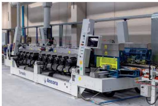
cess resulting in significant lower logistics and management costs and also maximised productivity (reaching numbers in the order of 20,000 m<sup>2</sup>/day). With the new laser system, the grinding process can be measured and controlled in real time, with automatic intervention in the event of errors, which guarantees continuous accurate grinding over time. All of this, of course, has advantages for the
