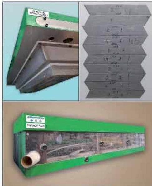
ISOSTATIC MONOCALIBER PLATE with 10 exits 75x450 CHEVRON, complete with mould and interchangeable and easy to replace liners at 45°, including a CARTER for dust extraction in GREEN ECONOMY technology, to increase the duration of the internal parts subject to wear due to friction with dust and to increase cleaning of the surrounding environment.
